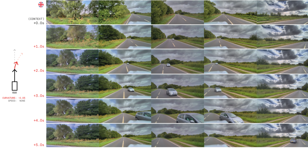
Figure 9: Ego-induced safety-critical scenarios. By applying unsafe action conditioning, GAIA-2 can generate hazardous situations, such as steering into oncoming traffic. We provide real video frames as context and GAIA-2 rolls out from these starting frames given some new action conditioning. In this example, we control the ego vehicle steering by conditioning on rightward curvature. We drop out speed so that GAIA-2 can generate multiple diverse outcomes. Note how the ego vehicle slows down while veering sharply into oncoming traffic. The oncoming vehicle swerves to avoid the ego vehicle.
