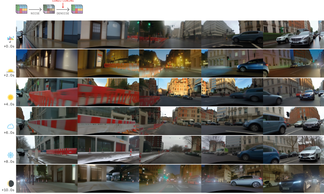
Figure 6: Augmentation through partial noising. By partially noising and denoising video frames, GAIA-2 transforms real video into diverse versions under different environmental settings, such as weather and time of day, while preserving semantic content and ego-actions.
