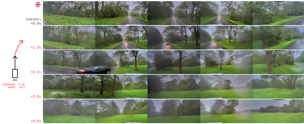
Figure 10: Extreme generalization behavior. When conditioned on high speed and strong curvature, GAIA-2 extrapolates off-road trajectories, capturing rare behaviors like driving into fields or forests.
