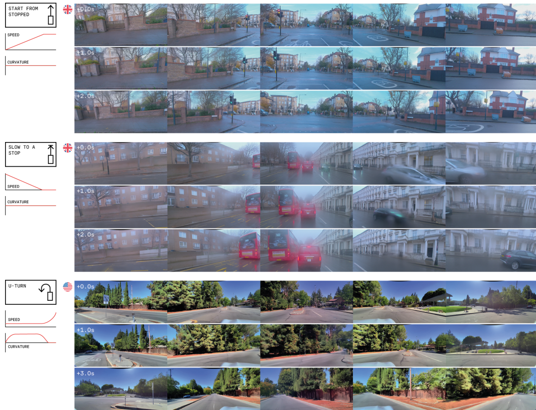
Figure 8: Action-based generation. GAIA-2 synthesizes diverse scenes from specified speed and curvature profiles. Each scenario is contextually plausible, despite the original video inputs being dropped out.
